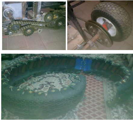
Fig.6 Mechanical hardware: sprocket chain, wheel, track
